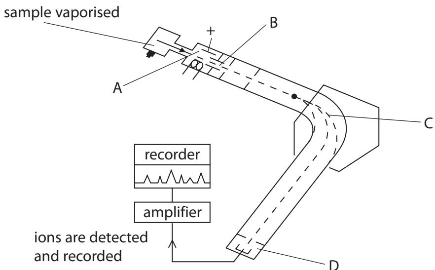
The region of the mass spectrometer in which ions are accelerated is
